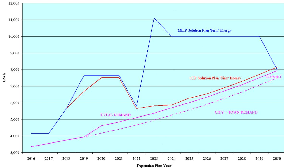
**Figure 2: Firm Energies of CLP & MILP Expansion Plans for the Development System**
