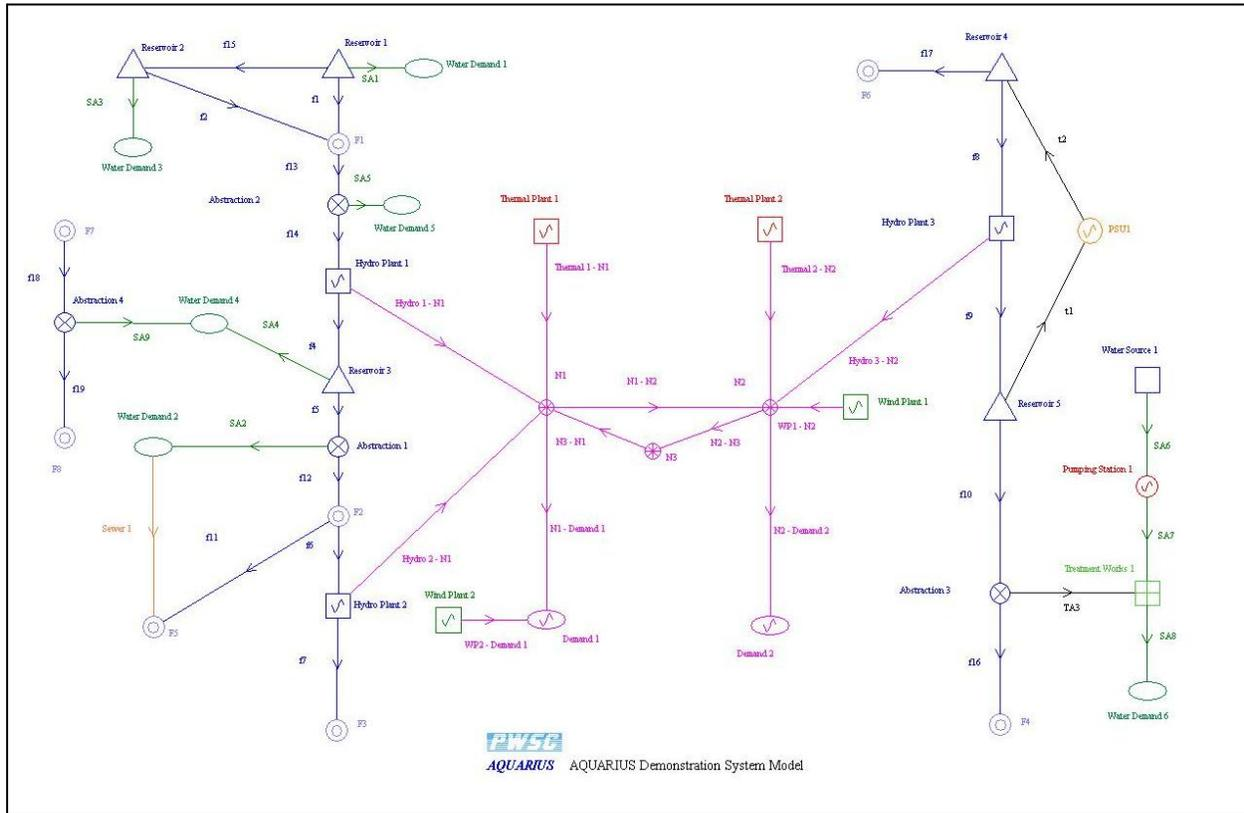
**Figure 1 : Water and Electricity Supply System Components Modelled by Program AQUARIUS**
